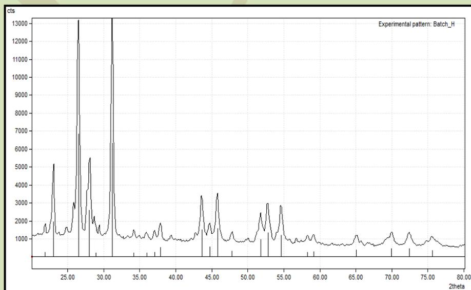
Figure2: Powder X-ray diffraction pattern of formulation
